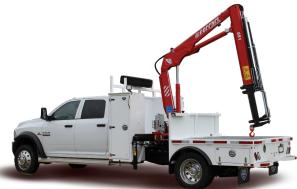
designed for oil and gas and pipeline contractors, picker decks are one of the most widely used crane truck packages in the industry.
